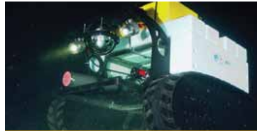
NEPTUNE Canada's "Wally", the world's first internet operated deep-sea crawler, will help researchers measure conditions at the sea floor.
