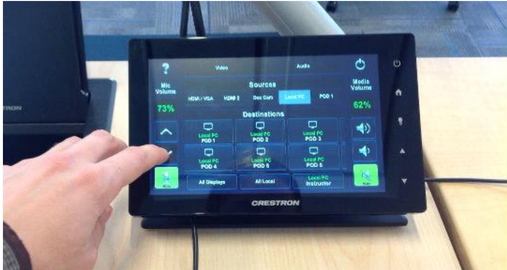
4. Mic volume controlled by Wireless Mic Volume on left side of touchscreen.
