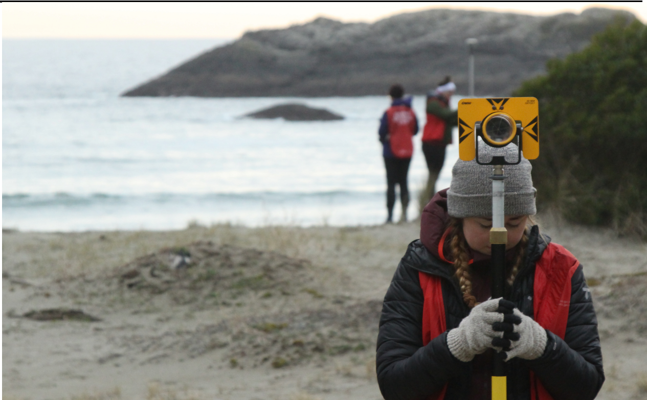
GIS data collection in action! Geography students surveying Schooner Dune System (2019) in Pacific Rim National Park Reserve. Multiple methods were used to create terrain surface models which were further used to detect change to this important ecosystem after winter storm season.
