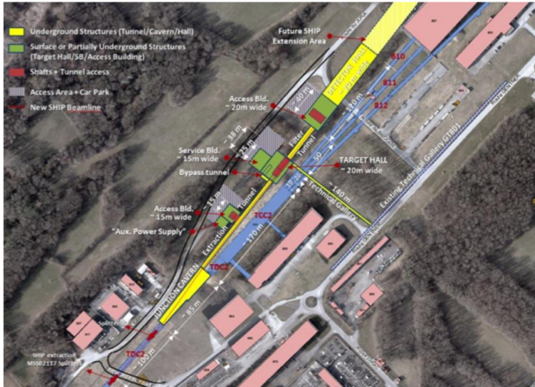
**Figure 20: Schematic layout of the civil engineering complex.**
