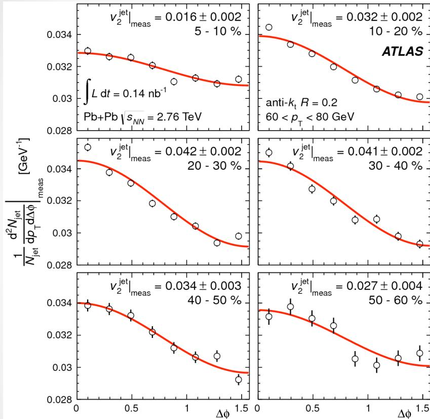
Azimuthal angle dependence of inclusive jet yields in Pb-Pb for 6 centrality ranges (curves are fits);  $v_2^{\text{jet}}$  measures single jet suppression as function of  $\Delta\phi$
