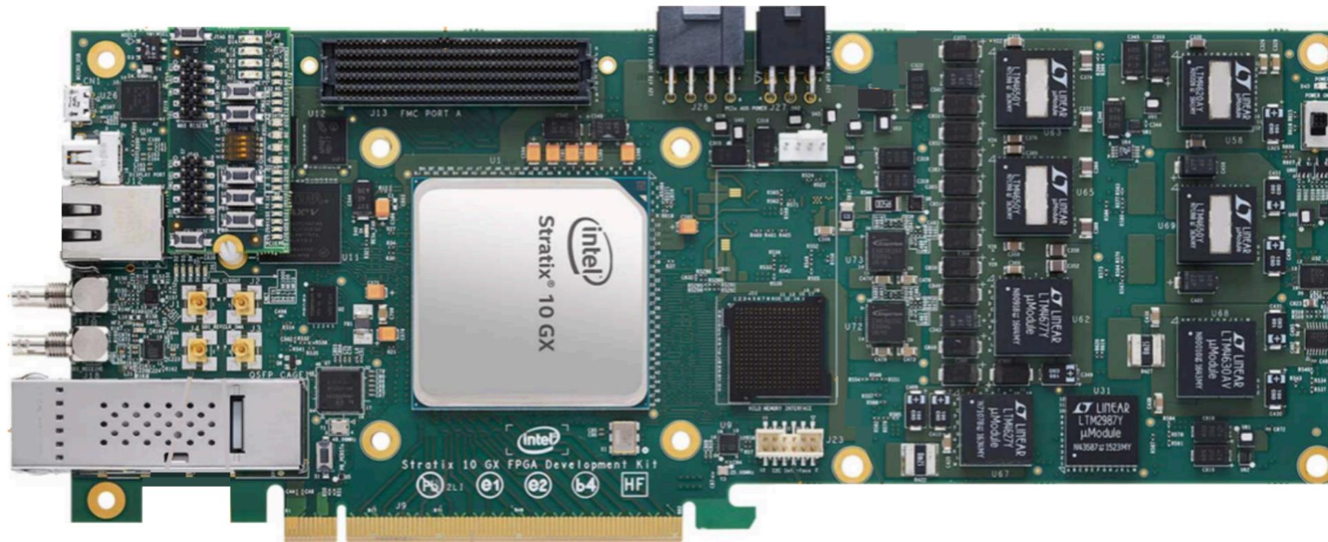
FIG 4: FRONTAL IMAGE OF THE INTEL STRATIX 10 GX BOARD [3]
