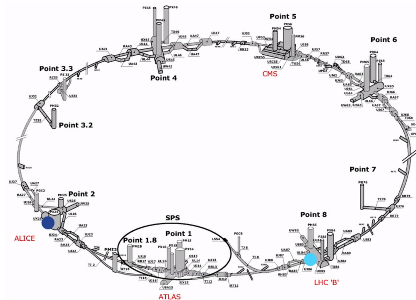
FIG 1: SKETCH OF THE UNDERGROUND LHC ACCELERATOR RING WITH ITS MAIN EXPERIMENTS [1]
