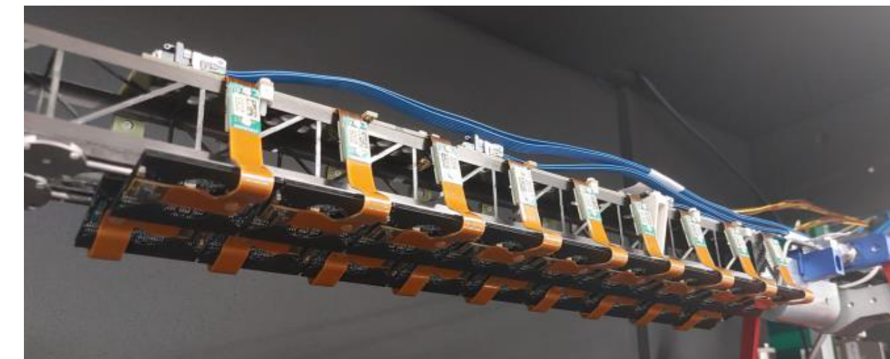
ITK pixel Pre-production loaded longeron
