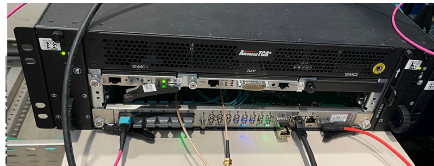
Integration between HGTD and new timing system (LTI) board
