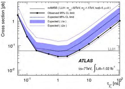
The observed and expected 95% CL upper limits on the signal cross section as a function of chargino lifetime for m(chargino) = 90.2 GeV
