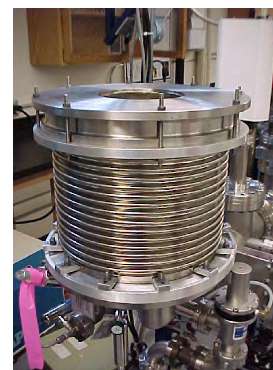
Bellows assembly during leak tests at UVic.
