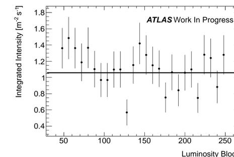
The cosmic muon integrated intensity for muons with transverse momenta above 20 GeV is measured almost 100 m underground to be constant at  $1.10 \pm 0.05$  (stat.)  $\text{s}^{-1} \text{m}^{-2}$ . This value is of the same order of magnitude as the approximated integrated intensity of cosmic muons with energies above 20 GeV at sea level of  $6.0 \text{ s}^{-1} \text{m}^{-2}$  in the range  $\theta < 75^\circ$ .
