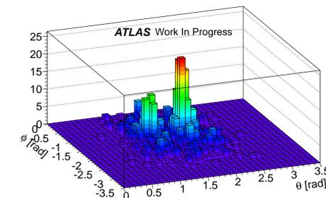
The two-dimensional histogram shows the number of muon candidates as a function of their directions in  $\theta$  and  $\phi$ . The distribution of the directions shows regions of higher integrated intensities (higher densities) where the two main access shafts are located and lower integrated intensities (lower densities) at shallower angles where there is more rock above to traverse.
