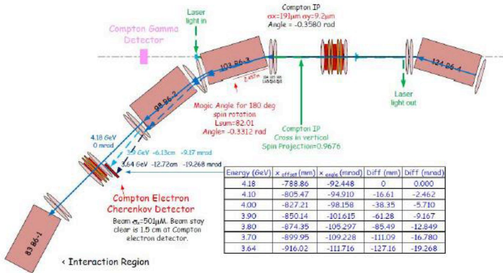
Figure 16.9: Layout of the Compton polarimeter.
