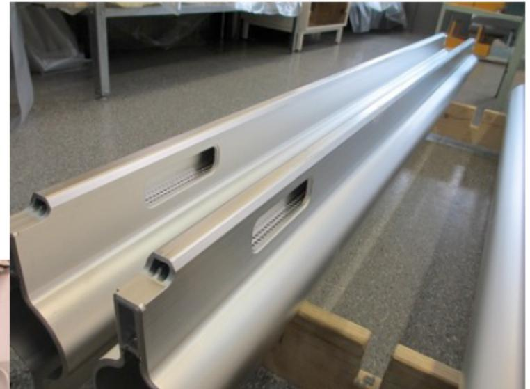
Beam pipe is made of aluminum.
