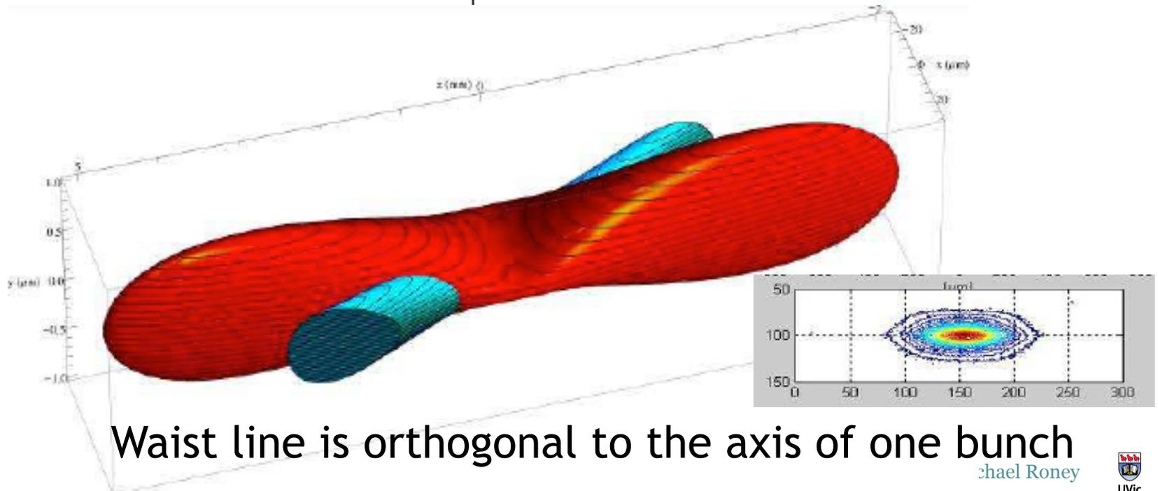
Waist line is orthogonal to the axis of one bunch
