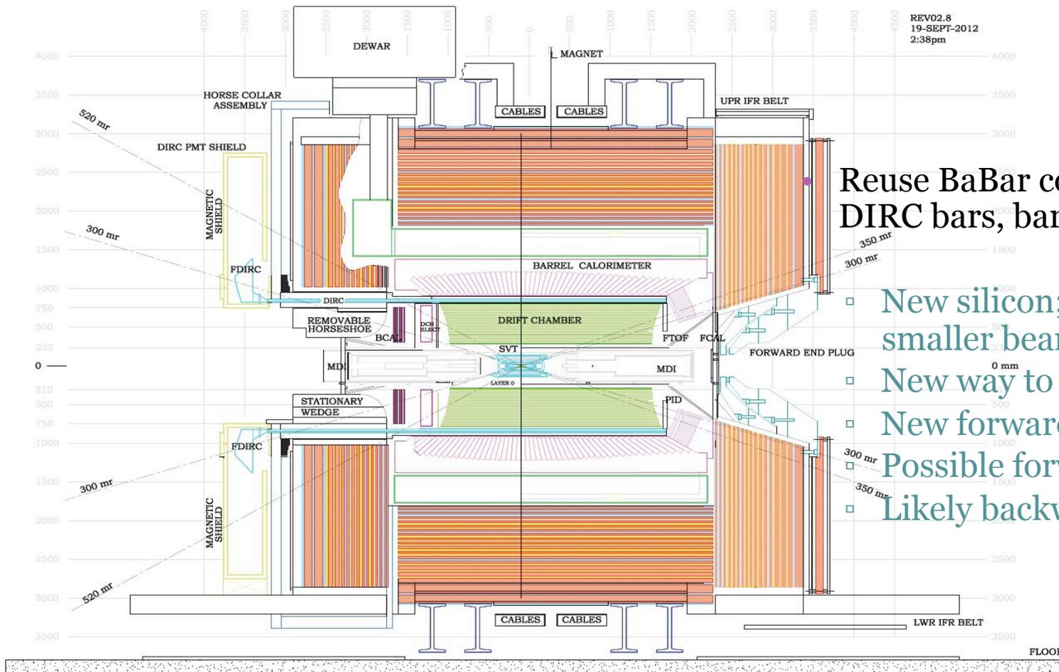
Reuse BaBar components: magnet, DIRC bars, barrel CsI calorimeter.
