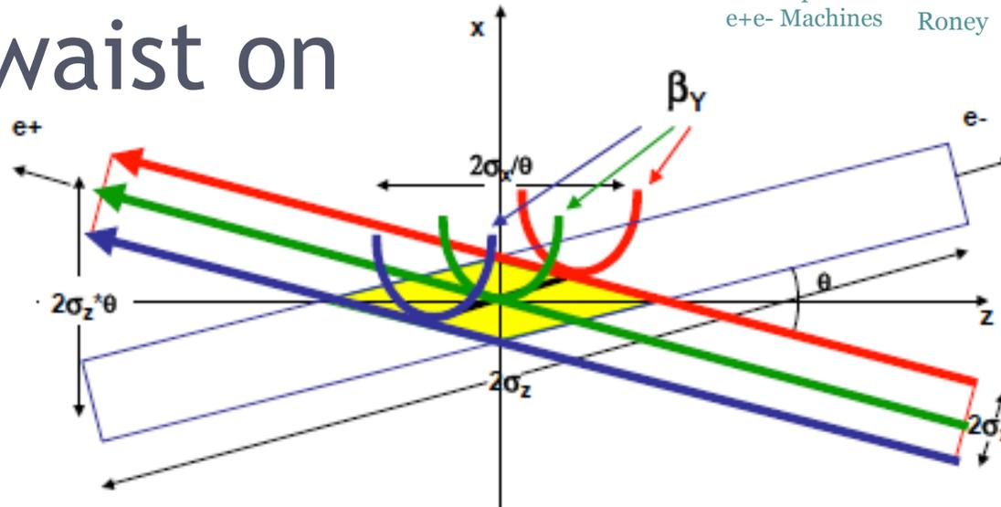
All particles in both beams collide in the minimum  $\beta_y$  region, with a net luminosity gain
