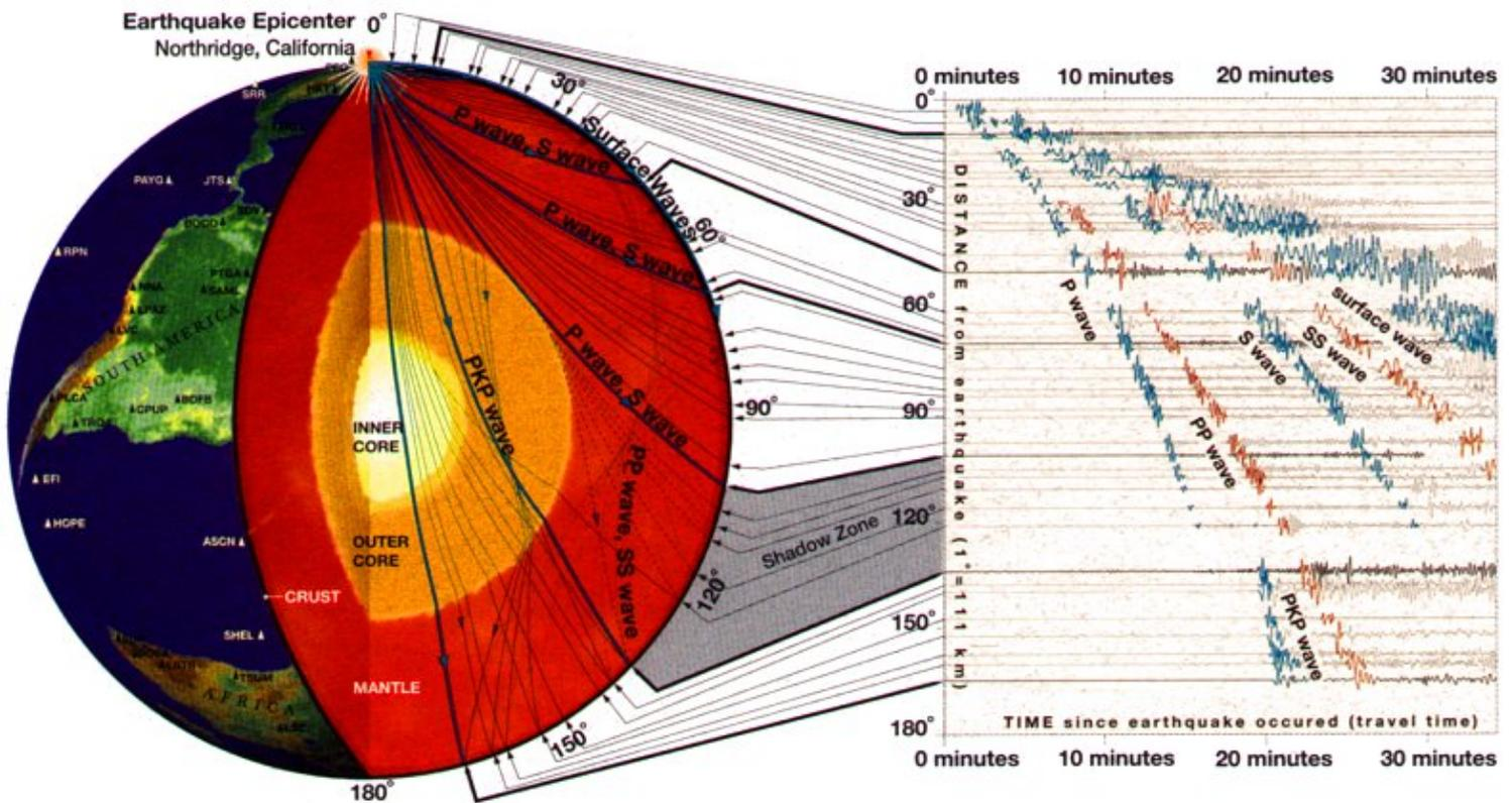
Example of geophysical remote sensing: Earthquake-generated seismic waves penetrate the earth and return to the surface, providing information on interior structure of inner core, outer core, mantle, and crust (IRIS Educational and Public Outreach Program, NSF EAR-1261681).
