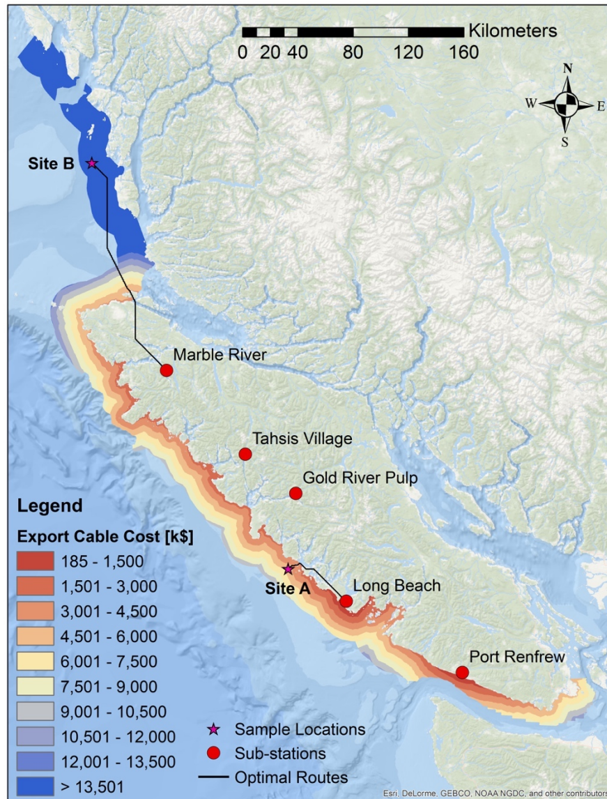
Figure 3.3 The cost distances to substations and the optimal cable routes.
