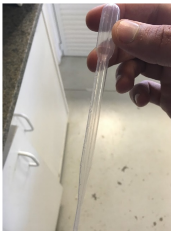
Figure 4.4: Liquid dropper used to insert solution of sulfuric acid inside the tube.
