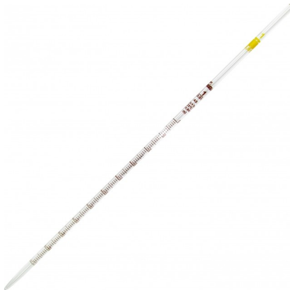
Figure 4.11: Example of 1ml graduated pipette used during charging procedure
