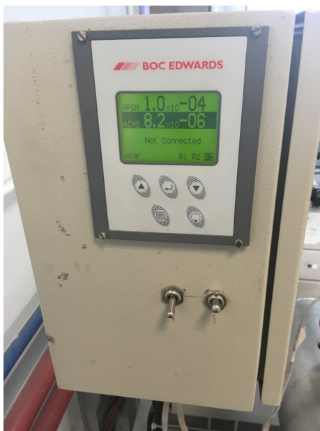
Figure 4.9: High vacuum pump display indicating pressure level in mbar
