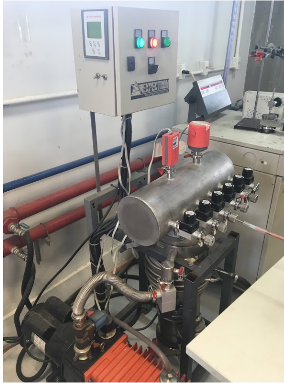
Figure 4.8: High vacuum pump in the lab
