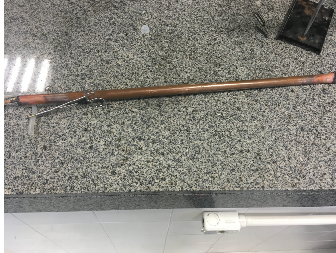
Figure 4.12: Thermosyphon filled with working fluid
