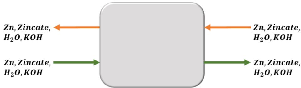
Figure 3.4: Fuel storage tank mass flows
