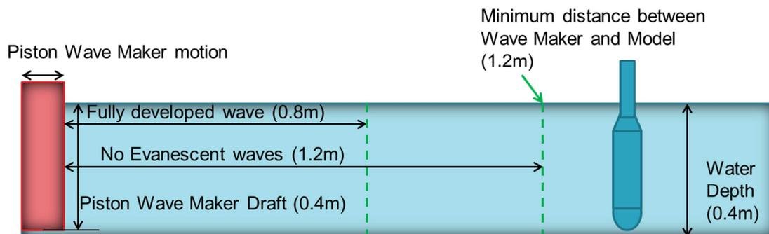
**Figure 11 - Test Facility Length Constraints**
