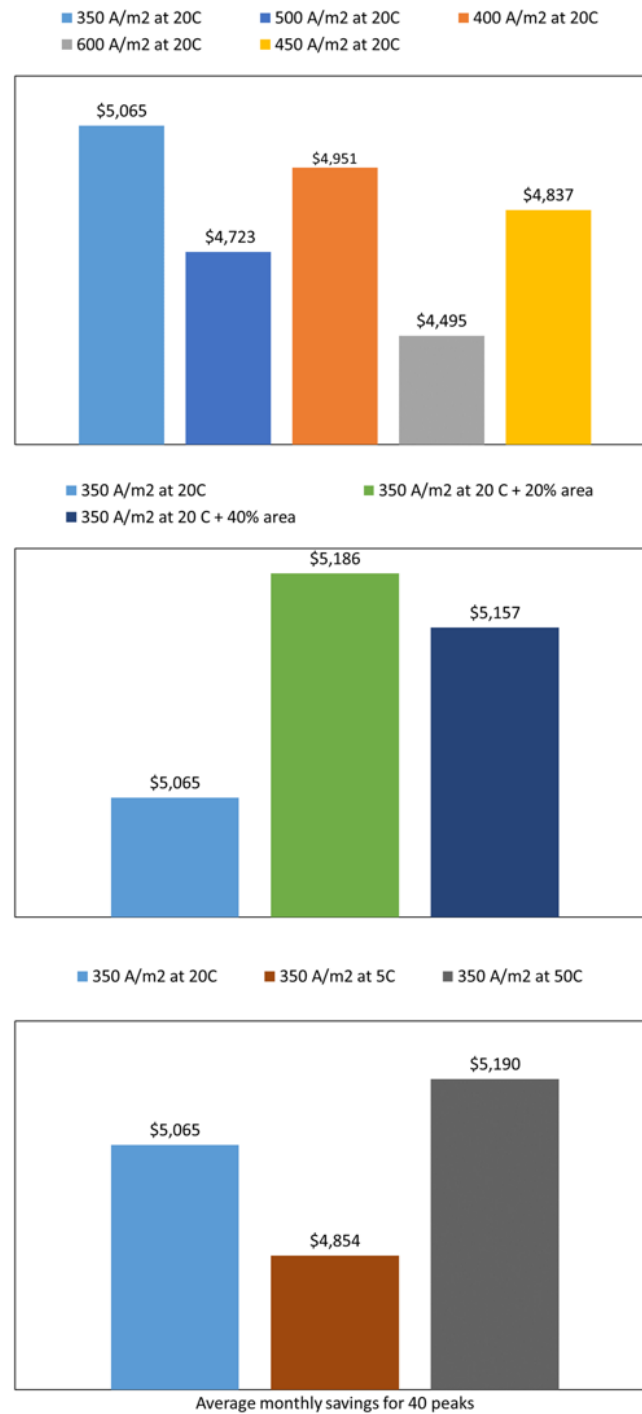
Figure 5.10: Average savings of the 500kW shaving the 40 highest peaks of each month, first plot have at different current densities, second plot different areas and third plot at different ambient temperatures
