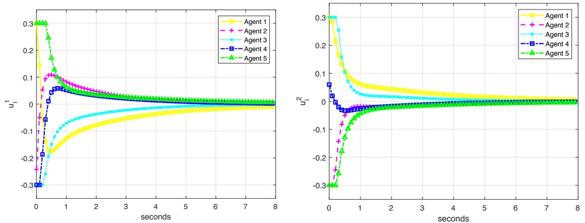
(a) MPC inputs for  $u_i^1$  coordinates(b) MPC inputs for  $u_i^2$  coordinates
