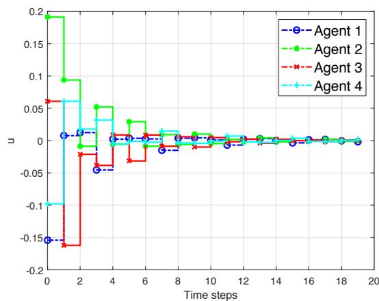
Figure 2.2: Control inputs of the linear consensus protocol
