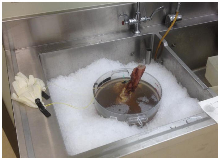
Figure 3-23: Specimen in fluid bath surrounded by ice for overnight storage between tests
