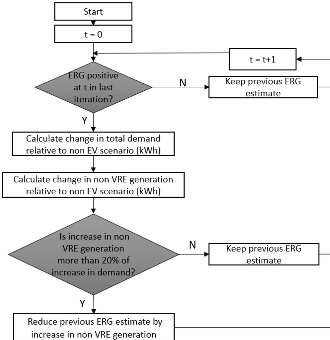
Figure 3: Flowchart for iterative procedure linking SILVER with charging model to ensure utility controlled charging only uses renewable generation
