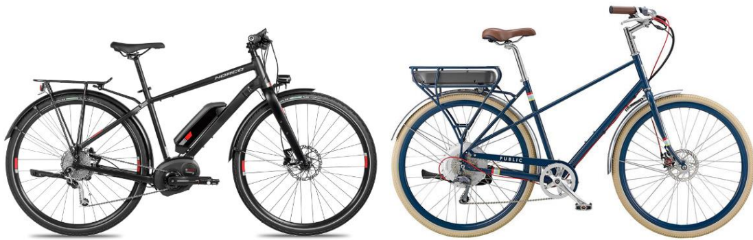
Figure 1: On the left, a typical Mid-Drive, geared motor E-bike, the Norco VLT as used in CRD E-bike Trial. On the right, a hub-located direct-drive e-bike. Images from www.norco.com and www.publicbikes.com
