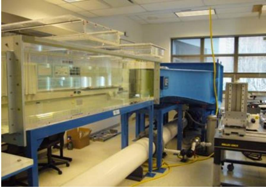
Fig. 1-4. The water channel at the Fluids Dynamics Research Laboratory at the Department of Mechanical Engineering of University of Victoria.
