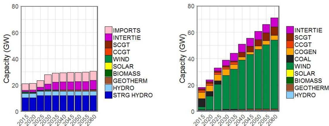
Figure 4-4: Installed capacity by type in British Columbia (left) and Alberta (right). Intertie refers to the BC-Alberta intertie. Imports refers to the capacity of the BC-US intertie.
