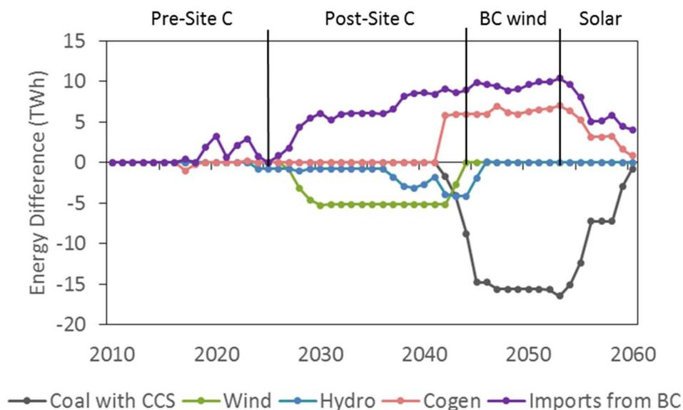
Figure 2-9: Difference in annual energy generation in Alberta between the 80% by 2050 carbon policy scenario with current transmission capacity (80%-C) and expandable transmission capacity (80%-E). Generation by coal with CCS, wind, hydro, cogeneration and imports from BC are shown. Positive values indicate higher generation in the expandable transmission capacity scenario.
