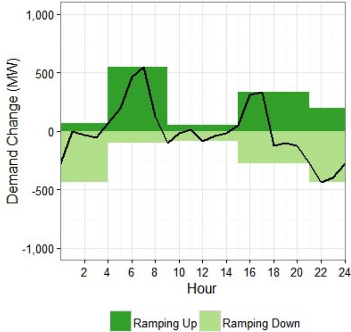
Figure 3-2: Hourly changes in demand (black line) and ramping demand for each time slice (green areas). Positive changes reflect ramp up requirements while negative changes are ramp down demand. Ramping demands for each time step is determined by the maximum up and down requirements.
