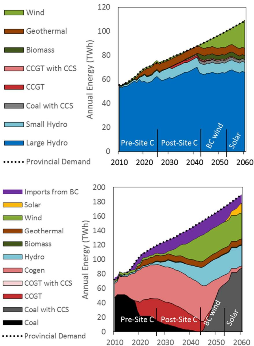
Figure 2-8: Stacked area plot of electricity generation in Alberta (top) and BC (bottom) from 2010 to 2060 in the 80% by 2050 scenario with expandable transmission capacity (80%-E). The dotted line indicates annual demand in the province; generation above this line is exported. Energy which is imported and resold is not included in this figure.
