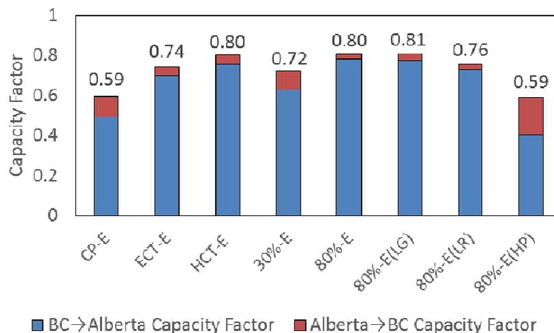
Figure 2-13: Stacked plot of the BC-Alberta intertie capacity factors in each scenario. The combined height is the total capacity factor of the intertie over the model period.
