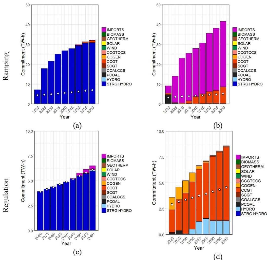
Figure 3-74: Unit commitment for flexibility service by generator for each demand in BC (left) and Alberta (right). Dots indicate service requirements based on load not including flexibility requirements from VR generation. Generators are stacked following the order in the legend.
