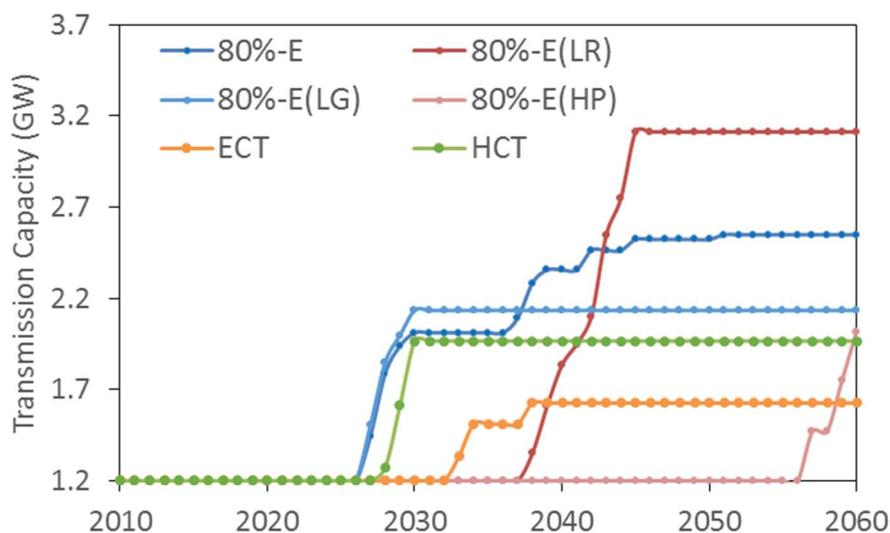
Figure 2-11: Optimal annual BC-Alberta intertie capacity for scenarios with expandable transmission. Intertie expansion does not occur in any scenario until the post-Site C era at the earliest. In the 80%-E(LR) scenario intertie expansion occurs in the BC wind era. In the 80%-E(HP) scenario intertie expansion occurs in the solar era.
