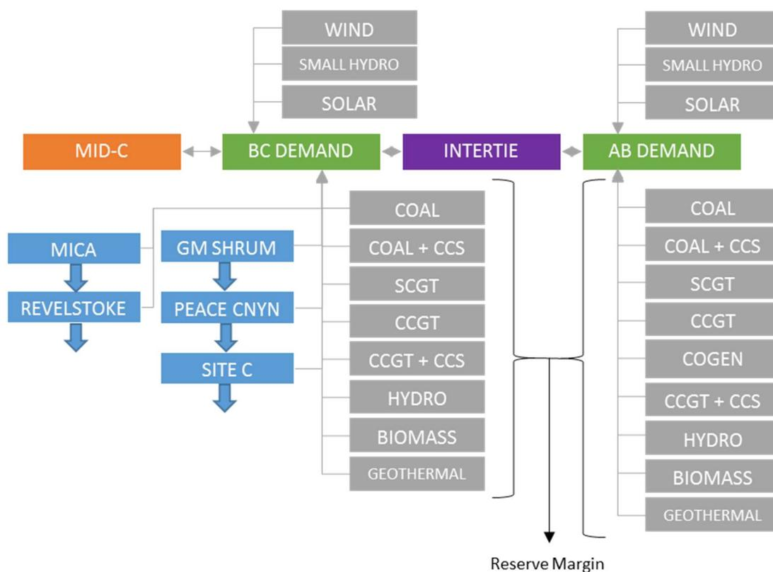
Figure 2-3: Diagram of the modelled electricity system. Electricity demand is shown in green, conventional generating units shown in grey, and cascaded hydro generators shown in blue. Grey arrows indicate power flows. Blue arrows indicate water flows.
