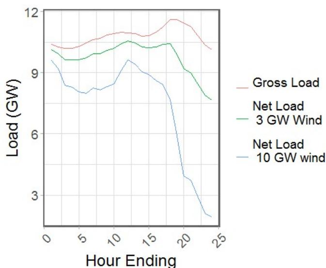
Figure 4-2: Net load profile for a sample day in Alberta with no wind (gross load), 3 GW of installed wind, and 10 GW of installed wind. With 3 GW of installed wind capacity, the load increase during the evening ramp-up is eliminated. Using the same wind profile but increasing the installed capacity to 10 GW, the evening ramp-up is replaced by a larger magnitude ramp-down.
