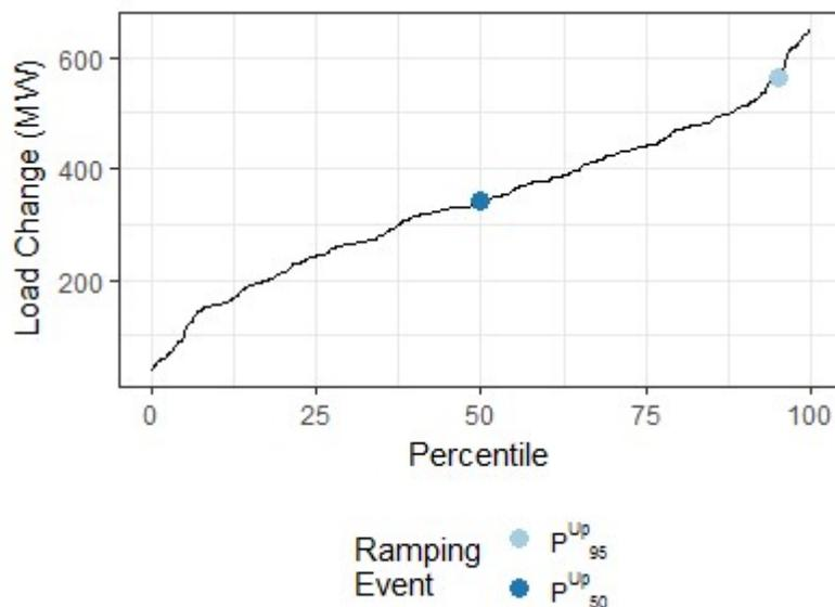
Figure 4-1: Hourly net load changes are sorted by magnitude. The 50th percentile of net load increases represents the  $P_{50}^{UP}$  demand. The difference between in 50th and 95th percentile represents the  $P_{95-50}^{UP}$  demand
