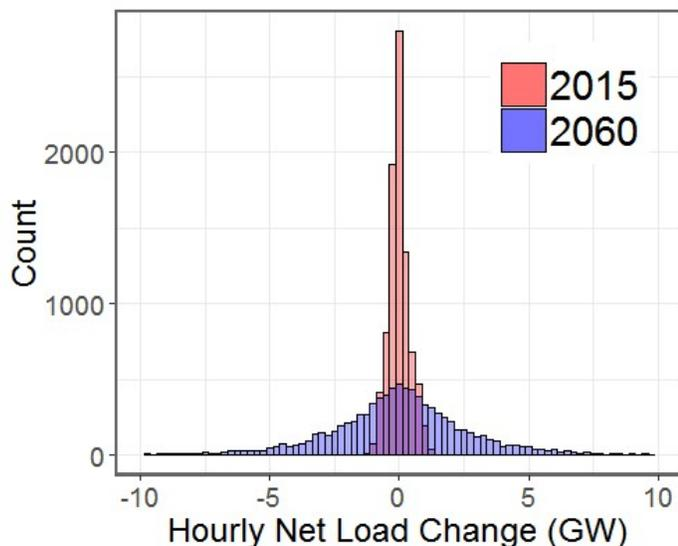
Figure 4-5: Histograms of hourly changes in the combined BC-Alberta net load in 2015 (red) and 2060 (blue). Net load refers to the hourly demand less generation from wind, solar, and small hydro.
