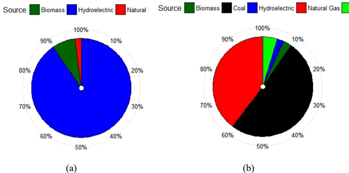
Figure 1-1: Electricity generation mixes in British Columbia (a) and Alberta (b) for 2015 [10]–[12]. British Columbia has an additional 242 MW of wind generation capacity for which the generation is not given in the source data. This generation is omitted from this plot and is estimated to roughly 2% of BC generation [10].
