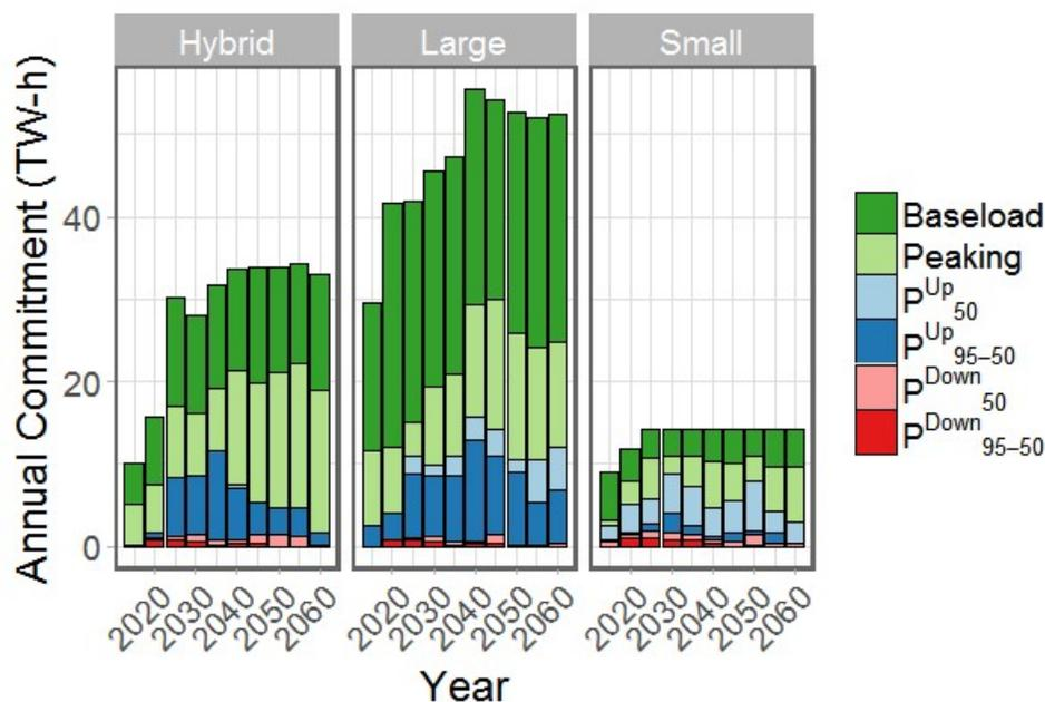
Figure 4-8: Annual commitment by type for storage hydroelectric generators in British Columbia. Generators are aggregated by storage type - large (GM Shrum, Peace Canyon, Mica), small (Seven Mile, Waneta), and hybrid (Site C, Revelstoke)
