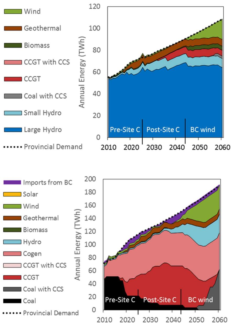
Figure 2-4: Stacked area plot of electricity generation in Alberta (top) and British Columbia (bottom) from 2010 to 2060 in the current policies scenario (CP-C and CP-E). The three *eras* are delineated in each graph. The dotted line indicates annual demand in the province; generation above this line is exported. Energy which is imported and resold is not included in this figure.
