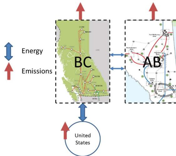
Figure 2-1: Diagram of the modelled area and connections between regions. Energy can flow between BC and both Alberta and the United States. Emissions are accounted for in all three regions.
