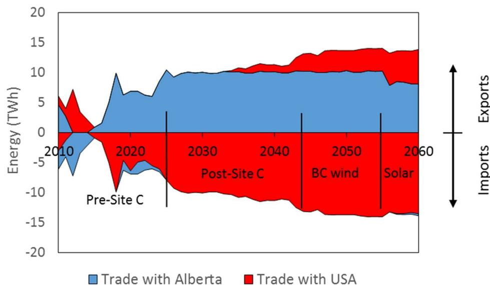
Figure 2-7: Stacked area plot of gross electricity trade between British Columbia and Alberta and the United States in the 80% by 2050 scenario with current transmission capacity (80%-C). Imports into BC are negative, exports from BC are positive. Total import volume to BC is 510 TWh. Total export volume from BC is 515 TWh.
