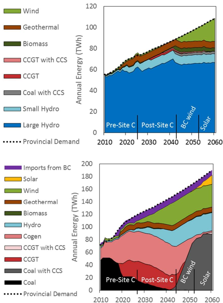
Figure 2-6: Stacked area plot of electricity generation in Alberta (top) and British Columbia (bottom) from 2010 to 2060 in the 80% by 2050 scenario with current transmission capacity (80%-C). The dotted line indicates annual demand in the province; generation above this line is exported. Energy which is imported and resold is not included in this figure.
