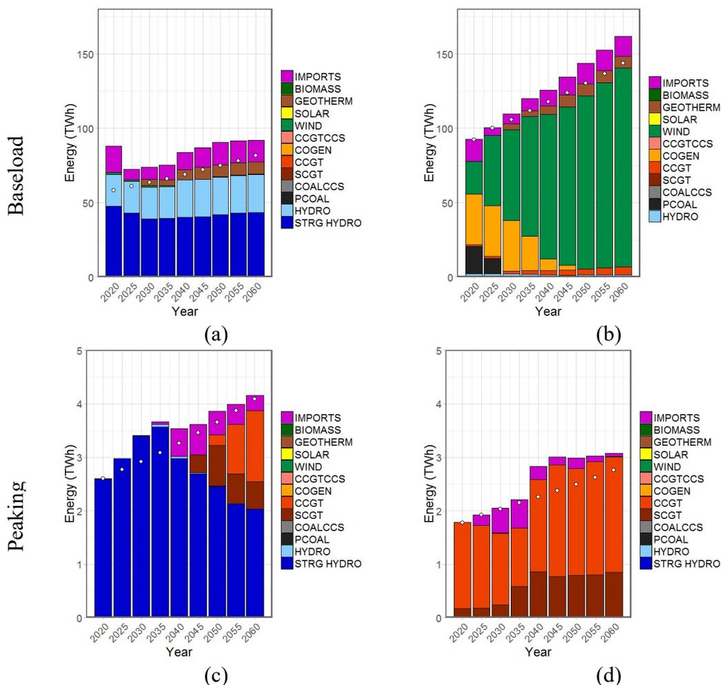
Figure 3-63: Energy production by generator for each demand in BC (left) and Alberta (right). Dots indicate service requirements based on load not including flexibility requirements from VR generation. Generators are stacked following the order in the legend.
