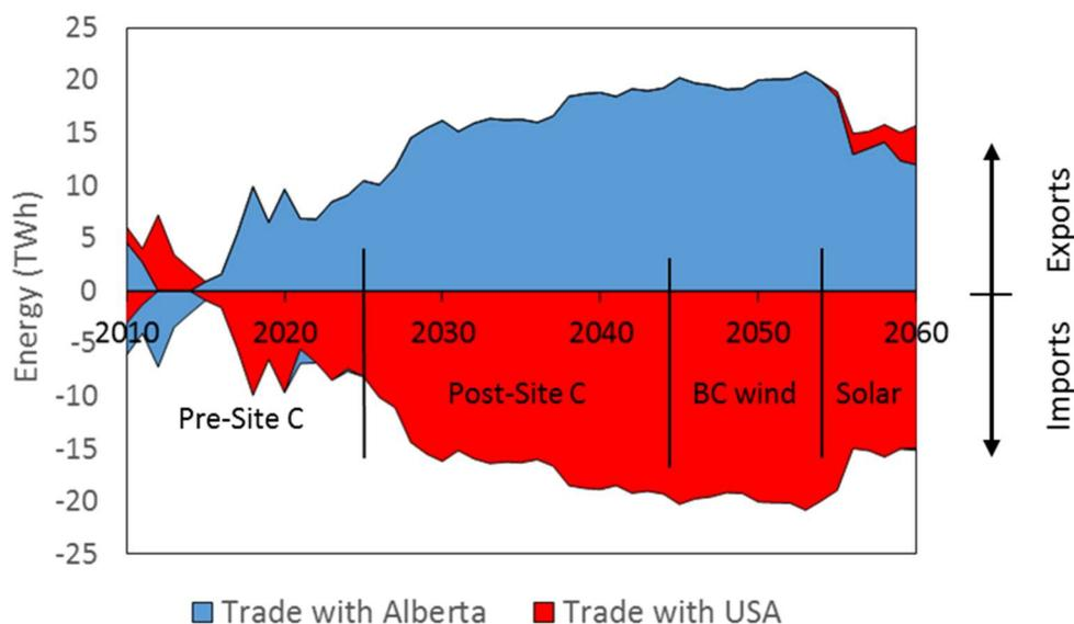
Figure 2-10: Stacked area plot of gross electricity exports from British Columbia to Alberta and the United States in the 80% by 2050 scenario with expandable transmission capacity (80%-E). Imports into BC are negative, exports from BC are positive. Total import volume to BC is 701 TWh. Total export volume from BC is 706 TWh.
