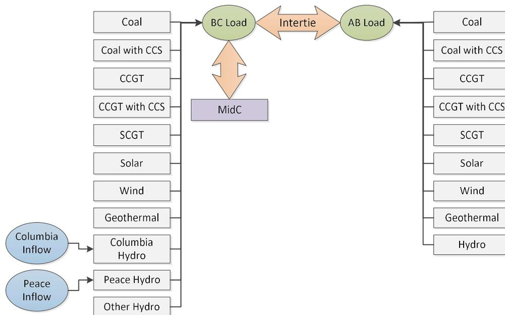
Figure 3-4: Schematic drawing of the BC-Alberta electricity system model. CCGT refers to combine cycle gas turbines, SCGT refers to simple cycle gas turbines
