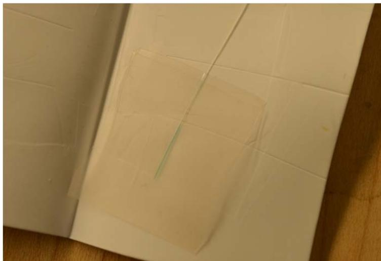
Figure 6-3: Embedded optical fiber sensing device within the Nafion<sup>®</sup> membrane.
