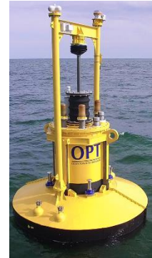
Figure 8: Ocean Power Technology's 11 PB3 PowerBuoy
