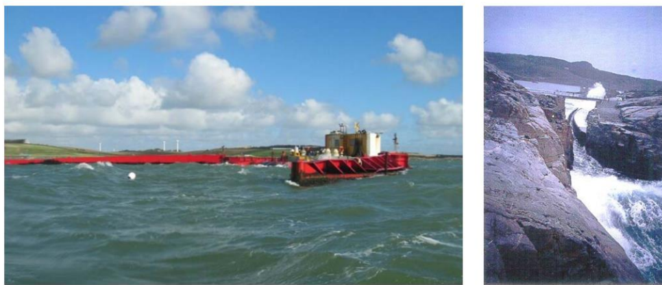
Figure 6: Visuals presenting two WEC designs operating under the overtopping principle: WaveDragon (left) and TAPCHAN 9 (right)
