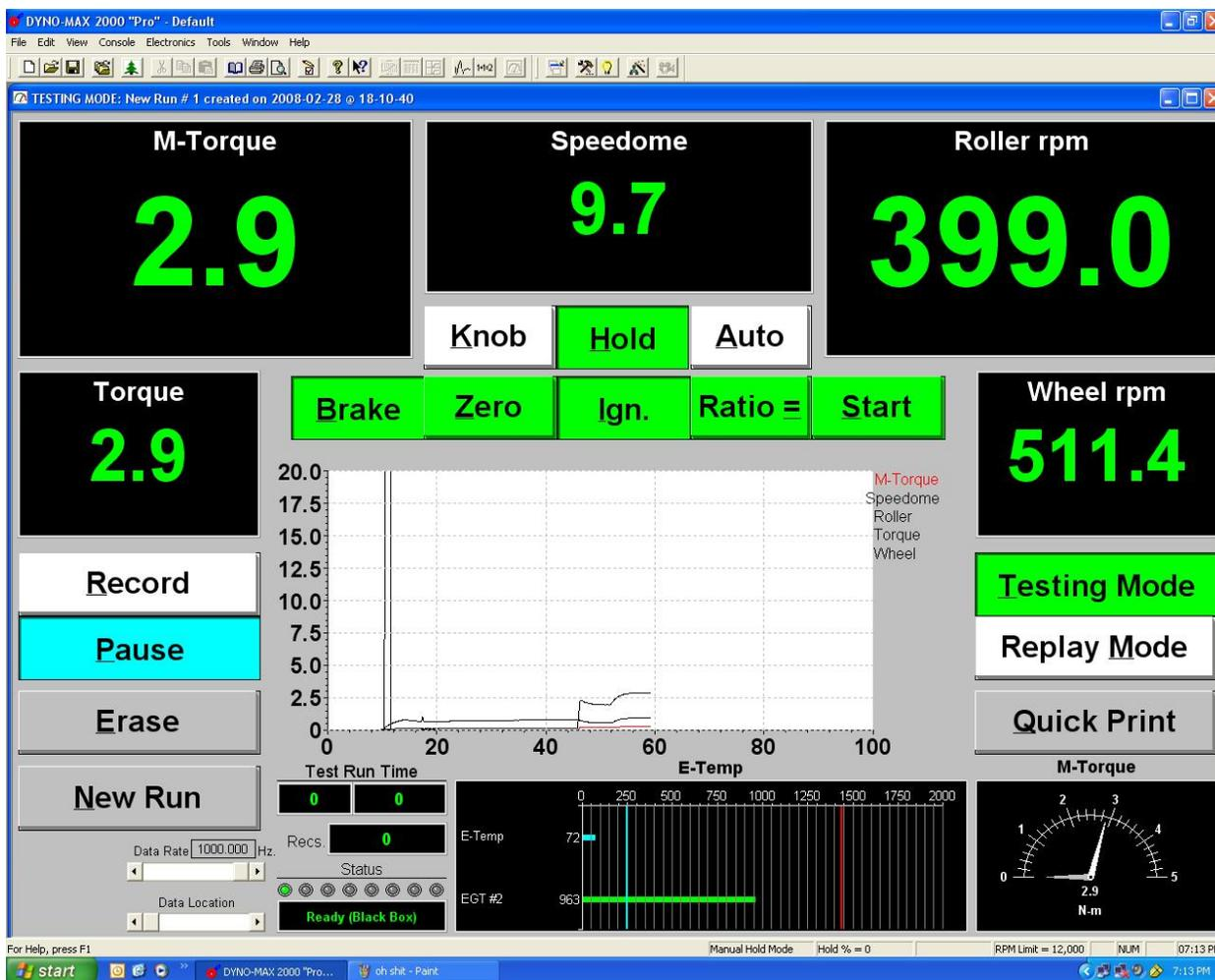
Figure 7-3. Test screen of the dynamometer computer software
