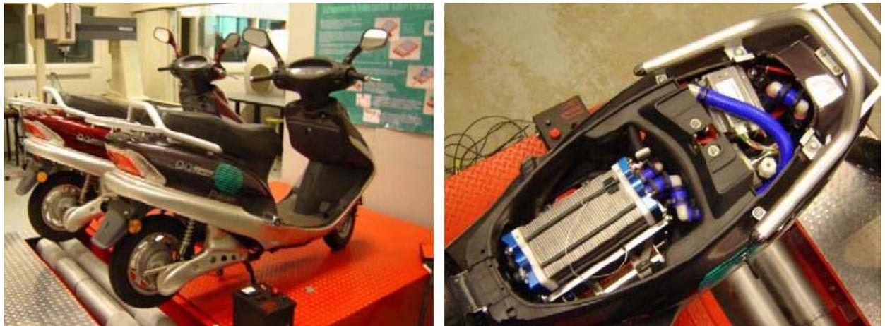
**Figure 7-2. Prototype low-speed vehicles and the fuel cell system of the fuel cell hybrid scooter**
