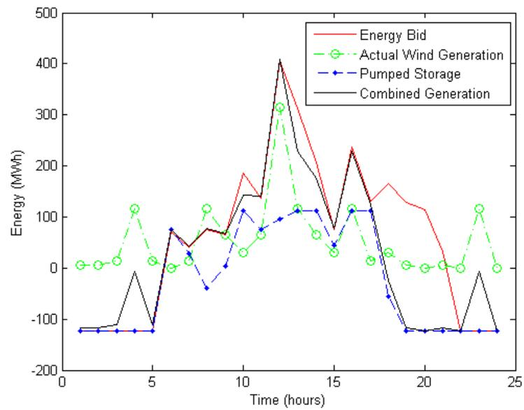
Figure D.6: Sample Day 5 Operation - Robust Case
