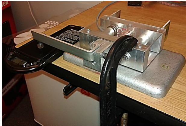
Figure 33 Set up for torque measurement
