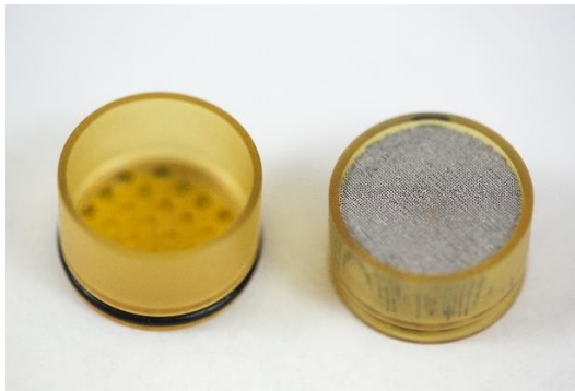
Fig. 13 Channeled microstructure puck and the puck housing designed for PM II cylindrical regenerators.
