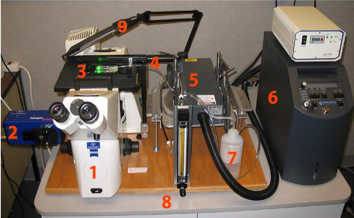
**Figure 2.15** Experimental apparatus. (1) Zeiss inverted microscope. (2) Cooled CCD camera. (3) Test section set into the stage of the microscope, coupled to the air flow line. (4) Beam expander (black). (5) Laser head. (6) Laser power supply and controller. (7) Bubbler humidifier. (8) Rotameter flow meter and control valve. (9) Fluorescent lamp.
