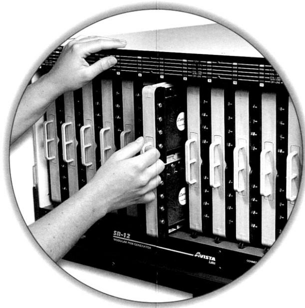
**Figure 1.3: One of the 720 W modules in Avista Lab's residential appliance.<sup>11</sup>**
