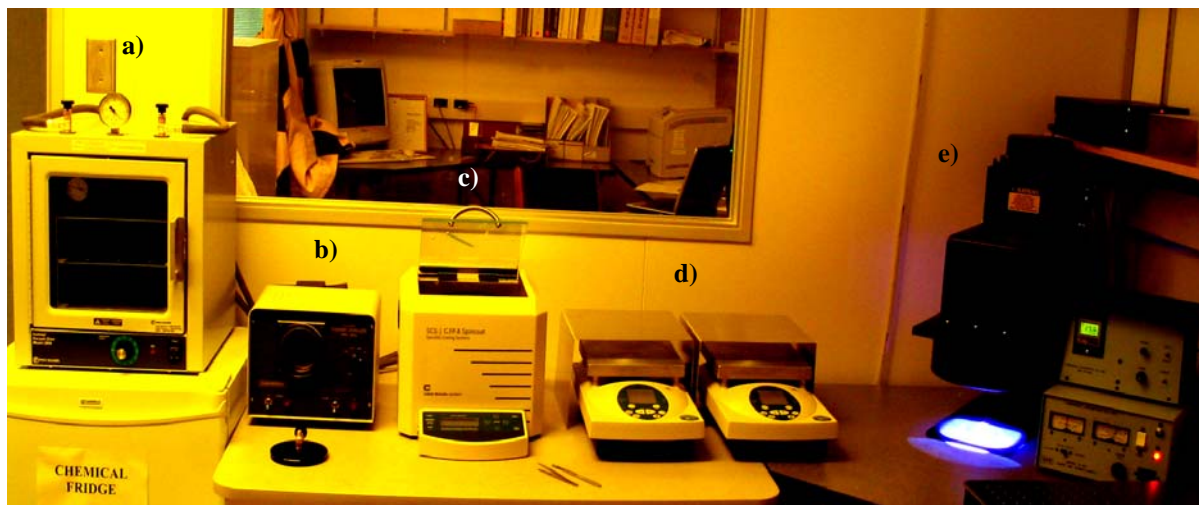
Figure 2.1 Microfabrication equipment in the microfluidics laboratory: a) vacuum oven, b) plasma cleaner, c) spin coater, d) digital hot plates, e) exposure unit, including power supply and timer. Ultrasonic cleaner is not pictured.
