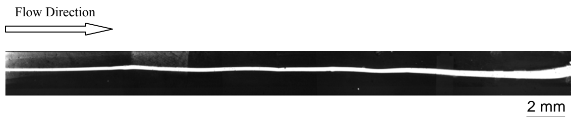
Figure 4.7 Composite image of in situ gold etching. Colaminar flow of gold etch solution sheathed by two water streams enters on the left and travels downstream. Broadening of the stream by diffusion is visible, as are slight distortions in the cross-stream location of the independent streams.
