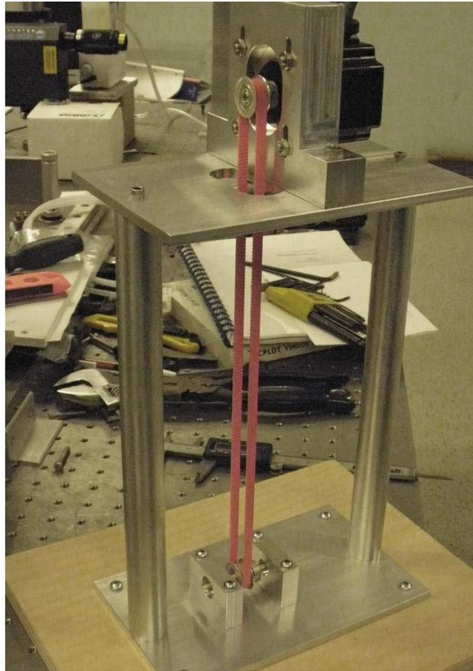
Figure 2.8: Rig for belt testing
