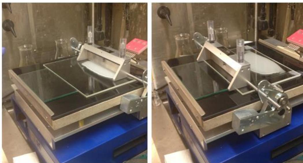
**Figure 3-19. D2020-TiO<sub>2</sub> solution on glass plate (left) and 1 mm film after casting (right)**
