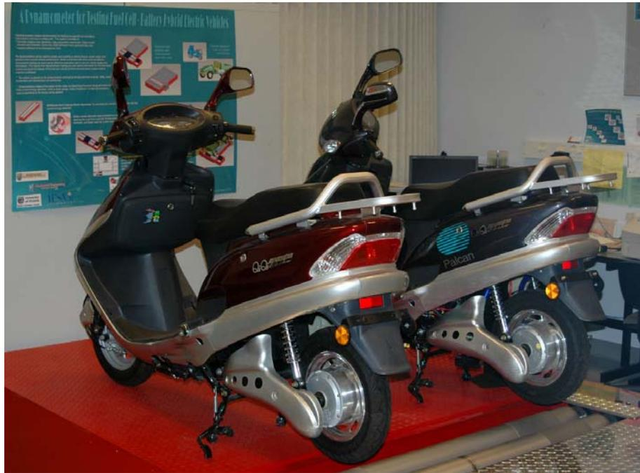
**Figure 6.1: Electric and FCHEV scooters on lab dynamometer**
