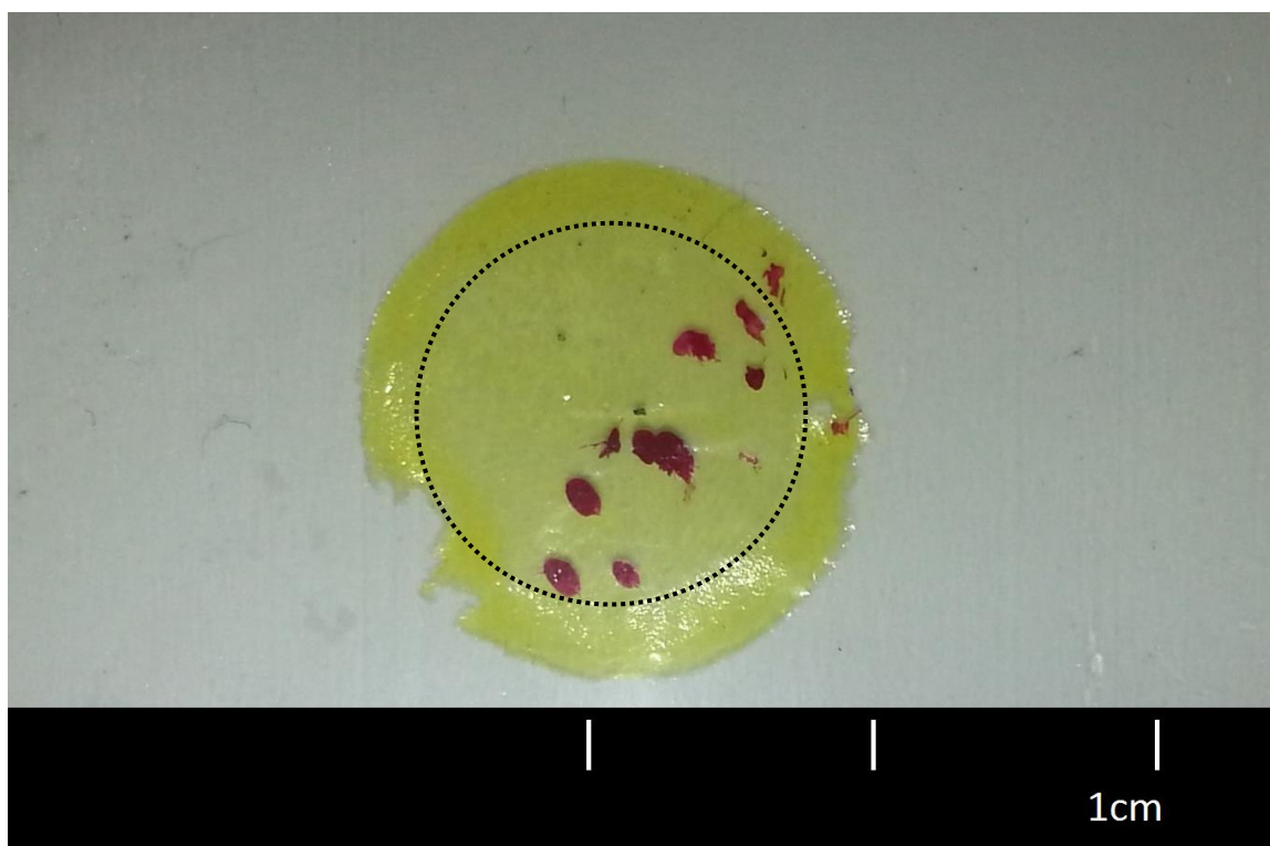
Figure 3.8: Dotted area indicating the outer boundary of the filtering surface area after O-ring compression. The cumulative area of the eight patches contained within the filtering surface area is subtracted to yield the reduced filtering surface area.
