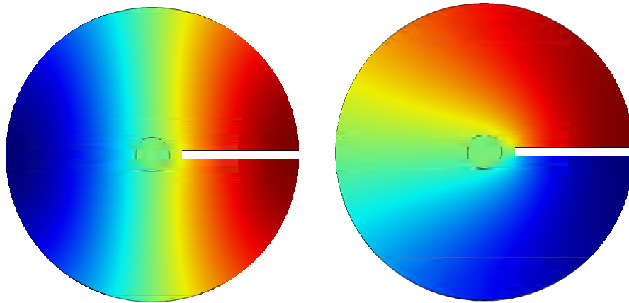
Figure 5.10: The mode shapes of the first acoustic diametral mode in the presence of the long splitter plate ( L_S = 81.4 mm): (a) f_A^1 = 998 Hz, (b) f_B^1 = 713 Hz.
