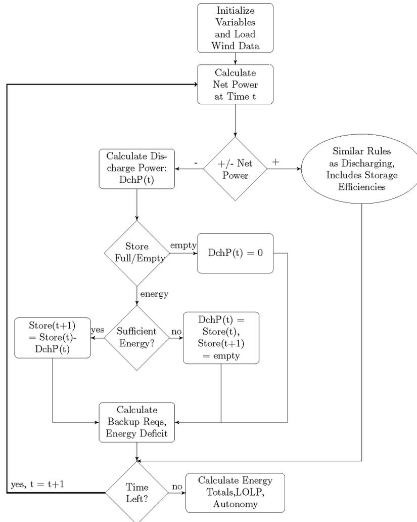
**Figure 8-1: Partial flowchart of time series testing function. The case of positive net power is neglected for simplicity.**
