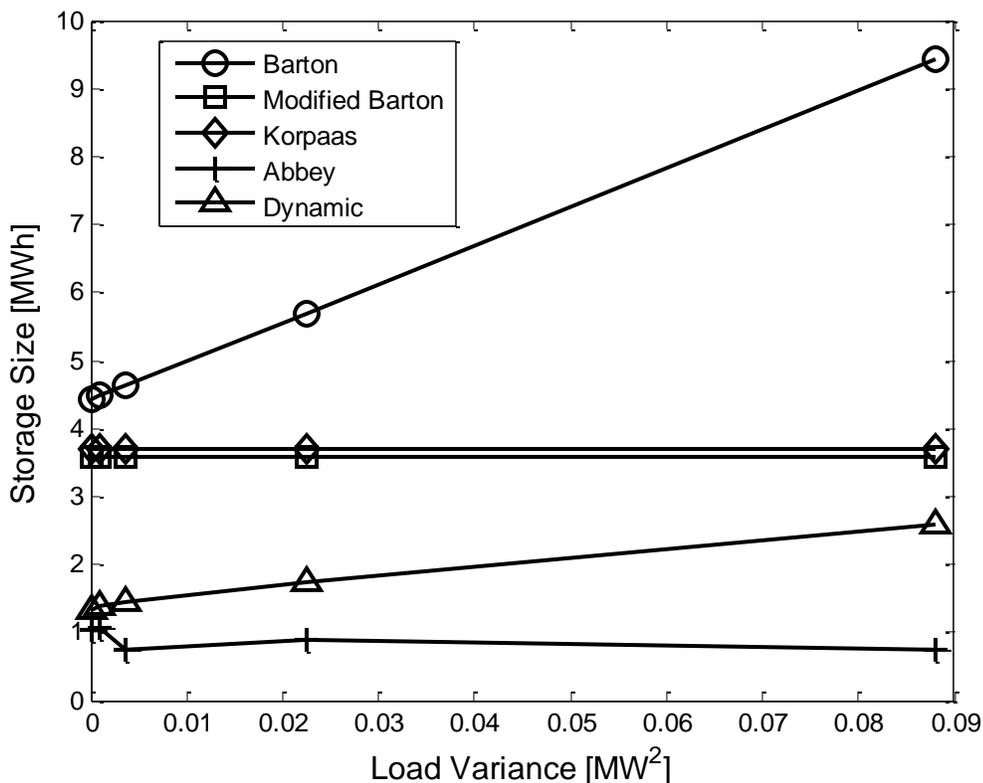
**Figure 5-8: Store size vs. variance for sinusoidal loads.**
