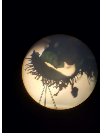
Close-up of lichen thallus showing the three ion-selective microelectrodes positioned next to the ventral surface of the lichen ready to measure ion flux
