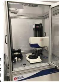
ZEEKO IRP 200 7-axis CNC optical polishing machine for producing ultra-precise surfaces on a variety of optical materials and surface forms. Used for post-polishing of components made on the Precitech Nanoform 250.
