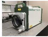
ESDI H2000 et Zygo interferometers Metrology instrument for non-contact precision measurement of flat or spherical surfaces.
