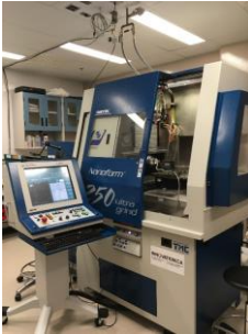
Precitech Nanoform 250 Ultra precision freeform CNC machine designed for single point diamond turning and freeform milling and grinding.
