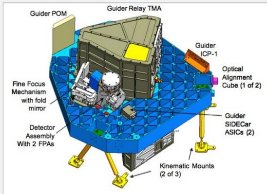
Figure 1: Diagram of the Fine Guidance Sensor optical components.<sup>1</sup>
