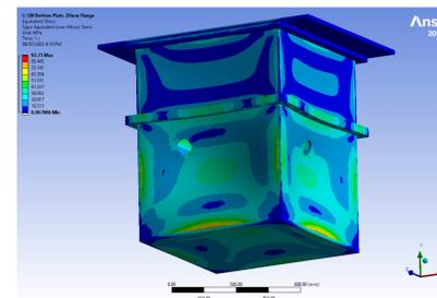
**Figure 2:** Finite element analysis showing the equivalent von-Mises stresses on the vacuum chamber walls due to a 1 atm pressure differential.
