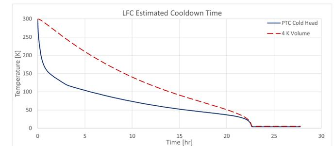
**Figure 3:** Time-dependent heat transfer simulation showing estimated cooldown time of the 4 K volume within the LFC. Blue: Pulse tube cryocooler cold head temperature. Red: 4 K volume temperature.
