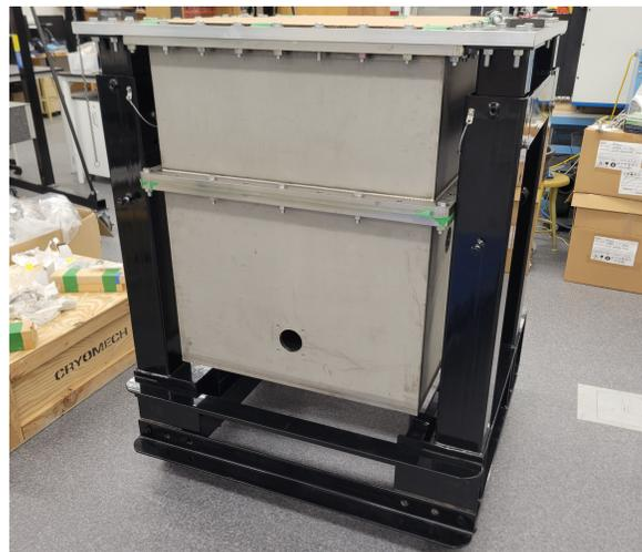
**Figure 4:** LFC vacuum chamber installed on supporting framework.
