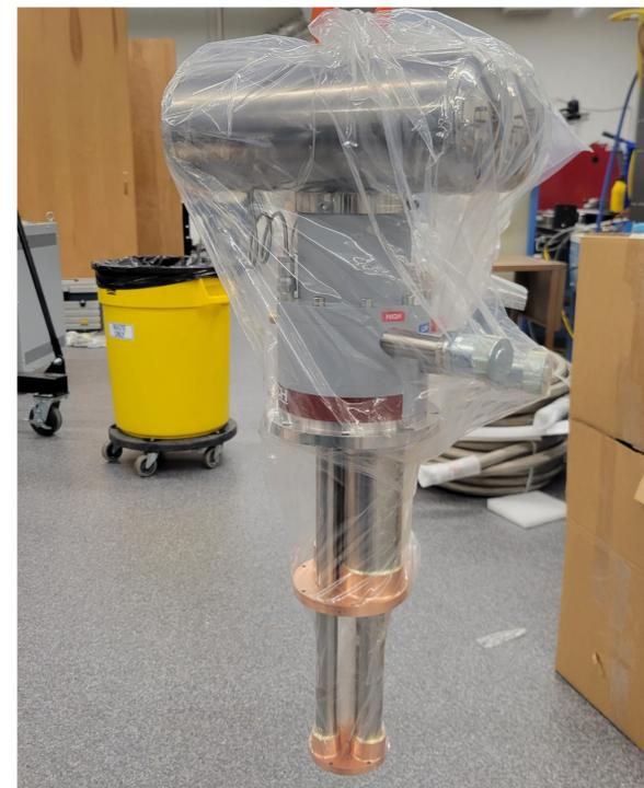
**Figure 7:** Cryomech PT415 pulse tube cryocooler. The Large Facility Cryostat is cooled by a pair of PT415 cryocoolers, each providing a cooling capacity of 1.5W @ 4.2K W/ 40W @ 45K [3].
