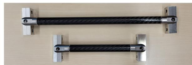
**Figure 6:** Assembled CFRP struts. Top: CFPR strut separating 45 K and 4 K stages of the cryostat. Bottom: CFRP strut separating room temperature vacuum chamber and 45 K stage of the cryostat.
