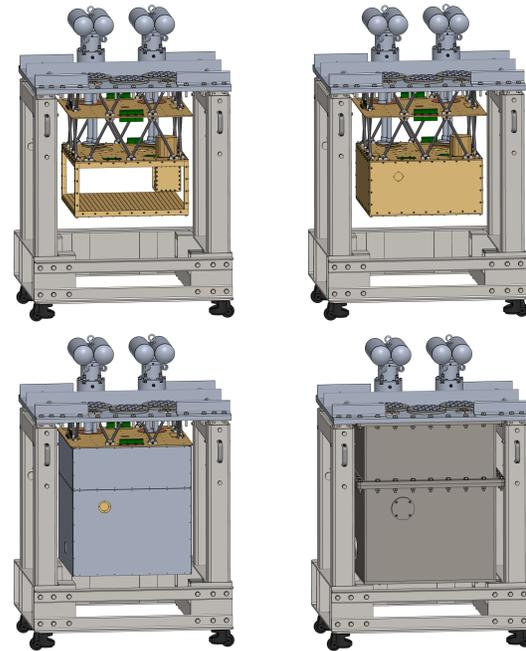
**Figure 1:** Overview of the Large Facility Cryostat. Two Cryomech PT415 pulse tube cryocoolers provide cooling capacity while carbon fiber reinforced polymer struts and concentric layers of radiation shielding reduce parasitic heat transfer. Top Left: Fully open. Top Right: 4 K radiation shielding. Bottom Left: 45 K radiation shielding. Bottom Right: Outer vacuum chamber.
