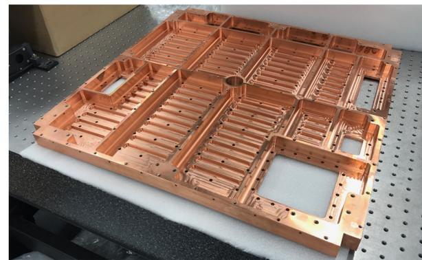
**Figure 5:** 4 K breadboard prior to gold plating. This breadboard is machined as a torsion box from a piece of billet copper and will be bolted to an upper skin (not shown) to increase rigidity.
