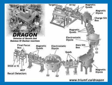
Located in the ISAC facility at TRIUMF in Vancouver, British Columbia, DRAGON is an apparatus designed to measure the rates of nuclear reactions important in astrophysics. Of particular interest are the reactions that made the elements around us; the nucleosynthesis reactions, which occur in the explosive environments of novae, supernovae and x-ray bursters.
