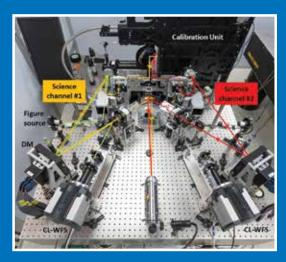
Raven has two science pick-off arms and three natural guide star wavefront sensors MOAO-correction is applied and the objects are remapped onto the Subaru Telescope's Infrared Camera and Spectrograph slit. *Credit: RAVEN team.*
