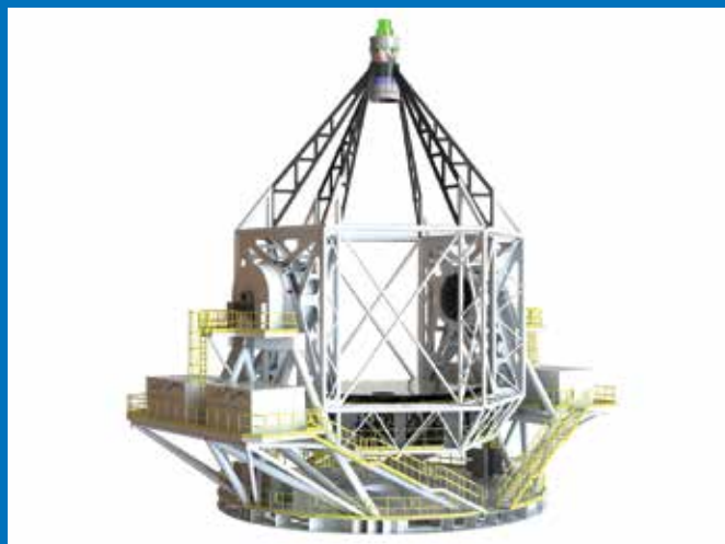
The conceptual design model of the MSE telescope. The hexagons that make up the primary mirror can be glimpsed just below the centre of the image.
