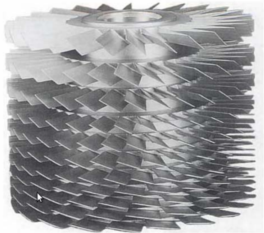
Fig. 11.9 Rotor used in a classical vertical turbomolecular pump. Reprinted with permission from Leybold Vakuum GmbH, Bonner Str. 498, 50968 Köln, Germany.
