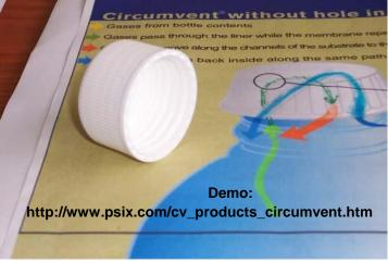
NOTE: The cap is designed to vent slowly and WILL NOT release pressure from an instantaneous reaction. USE PRUDENT PRACTICES AND GOOD JUDGEMENT! If you are pouring acid waste always wear proper personal protective equipment and work in a fume hood. If you expect an immediate reaction, let the materials react and vent before affixing and tightening the cap
