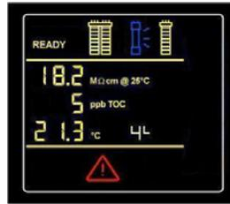
**System Alarms** When an Alarm is shown, it is listed under the System Alarms LCD. See the section <View Operation> for information on how to access this LCD.
