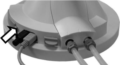
A photograph of the Q-POD Base, a white, circular device. On the left side, there are two PS/2 ports. A black Termination Plug is inserted into the top PS/2 port. A white arrow points to the plug. To the right, there are two other ports with cables plugged into them. |
