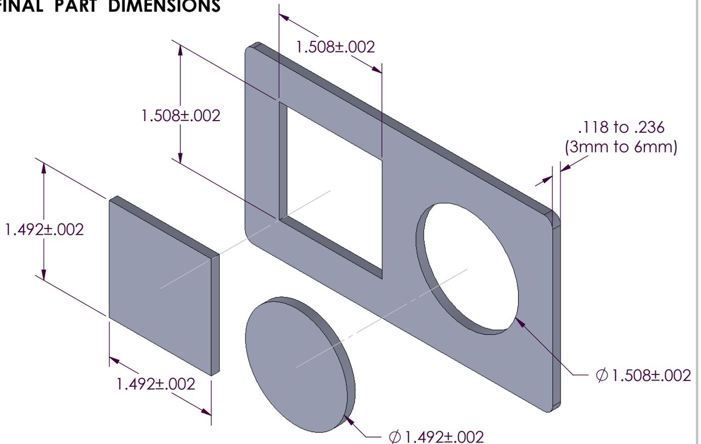
WIDTH OF CUT (KERF) IS 0.008", SO FEMALE CAVITIES ARE 0.008" LARGER THAN DRAFTED, AND MALE COUNTERPARTS ARE 0.008" SMALLER THAN DRAFTED (0.004" ON EACH SIDE)
