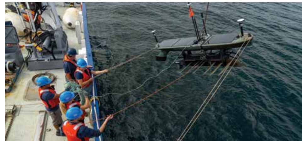
ONC deploys the Liquid Robotics wave glider, an autonomous floating platform that collects oceanographic data—part of ONC's pioneering seafloor geodesy monitoring system. CREDIT: OCEAN EXPLORATION TRUST
